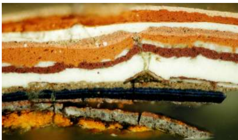
Cross section of a paint sample from Hinemihi's maihi (bargeboards) showing the longest paint sequence
